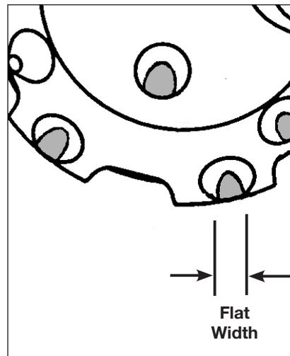
Face buttons which are flat generally indicate a lack of hammer blow energy or insufficient thrust.
