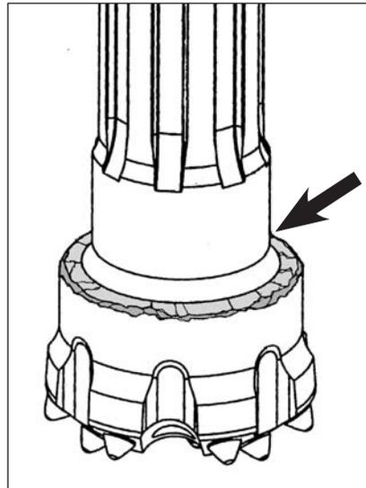
Shank breakage across the splines is generally caused by using a worn chuck, excessive torque or incorrect use of oversize drill bits.
