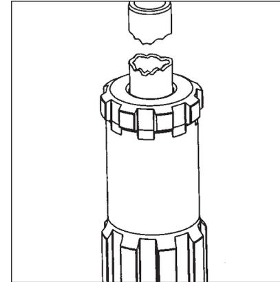
Inspect the striking end for damage or corrosion, generally caused by lack of lubrication or foreign particles caught between the piston and striking end
