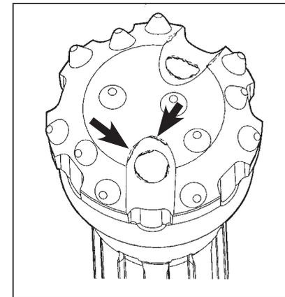
High levels of body wash and energy produced by the piston striking the drill bit can cause buttons to be hammered out of the bit body. This is known as button 'pop-out'. Button 'pop-out' can also occur even in drill bits with little body wash, where drilling in very soft conditions is being carried out and constant flushing is necessary because the drill bit face is not in constant contact with the bedrock.
