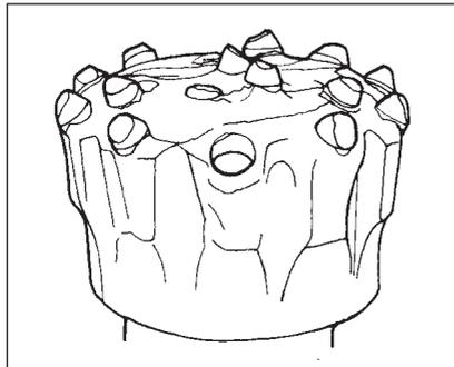
If the head is unevenly worn, the most likely causes are incorrect regrinding, bent drill tubes or drill string not being centralised in the drill rig table
