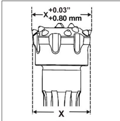
In highly abrasive conditions, the metal may wear more quickly than the carbide inserts. This is known as 'body wash' and in order to minimise carbide breakages, the carbide should be ground so that it does not protrude more than 9 mm (0.35") above the metal surface.
