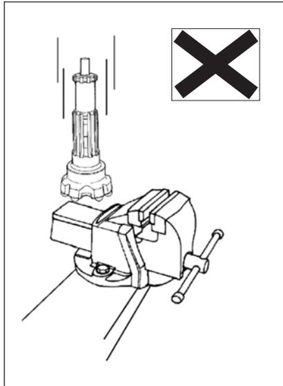
Do not allow tungsten carbide buttons to come into contact with each other.
