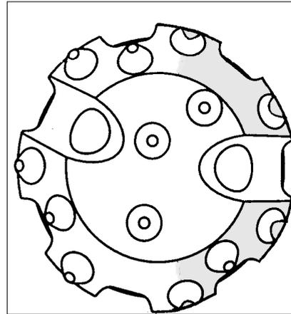
Excessive feed force can cause cracks on the face of the drill bit which can lead to large pieces of metal breaking off.
