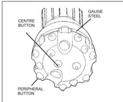
New tungsten carbide inserts work in compression where they are strong. As the carbide wears, flat spots appear leading to a horizontal or 'shear' load on the button
