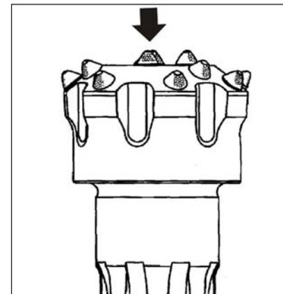
Broken inserts are generally caused by overdrilling the drill bit before reconditioning, reaming the hole, using excessive feed force or where there are existing tungsten carbide or other metal particles in the hole.
