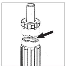
Damage to the shoulder is usually caused by excessive or insufficient thrust.
