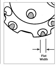
Face buttons which are flat generally indicate a lack of hammer blow energy or insufficient thrust.
