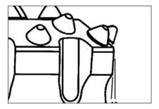
Ensure that the depth of flushing grooves is adequate and re-grind them regularly to allow free evacuation of the drilling debris.
