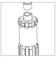
Inspect the striking end for damage or corrosion, generally caused by lack of lubrication or foreign particles caught between the piston and striking end
