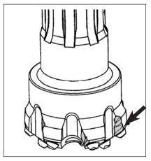
The depth of flushing grooves must be monitored as abrasion and/or high rpm wears away the drill bit body. The grooves must be regularly ground to ensure that drilling debris can adequately escape.
