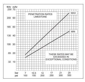
Penetration rates are generally dictated by air pressure. The higher the air pressure, the faster the hammer will drill.
