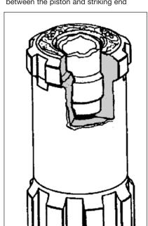
Ensure that the foot valve is not broken. This is generally caused by a worn piston or cylinder bore causing misalignment, lack of lubrication causing pick-up or corrosion by water.
