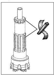
Shank breakage across the shank retaining ring diameter is generally caused by lack of lubrication or worn bit retaining rings, bit guide bush or bottom spacer.
