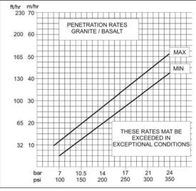
For example, if a hole diameter of 165 mm (6.1/2") was needed and a penetration rate of 30 m/hr drilling in granite. an air pressure of around 17 bar (250 psi) would be necessary.
