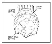
New tungsten carbide inserts work in compression where they are strong. As the carbide wears, flat spots appear leading to a horizontal or 'shear' load on the button
