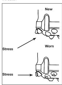
In abrasive conditions, it is advisable to monitor the rate of wear over a measured depth drilled to determine the frequency of re-grinding necessary. It is recommended that flat widths should generally not exceed 25% of the button diameter although this varies from manufacturer to manufacturer.
