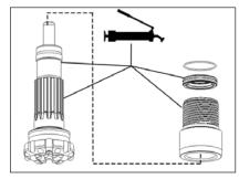
Inspect the drill bit, before use for any damage which may have occurred during transportation and prior to commissioning, take a note of the drill bit part number and serial number for future reference.
