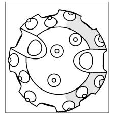
Excessive feed force can cause cracks on the face of the drill bit which can lead to large pieces of metal breaking off.
