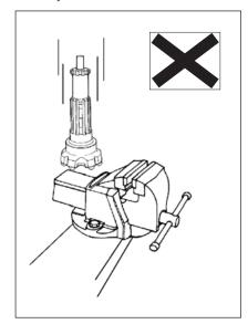
Do not allow tungsten carbide buttons to come into contact with each other.
