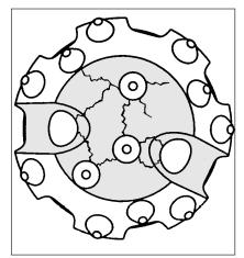
Re-drilling caused by poor hole cleaning and also high abrasion can result in deformation around the edges of exhaust holes and flushing grooves. These should be ground to ensure a clean obstruction free passage for exhausting air.
