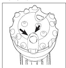
High levels of body wash and energy produced by the piston striking the drill bit can cause buttons to be hammered outof the bit body. This is known as button 'pop-out'. Button 'pop-out' can also occur even in drill bits with little body wash, where drilling in very soft conditions is being carried out and constant flushing is necessary because the drill bit face is not in constant contact with the bedrock.
