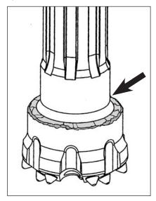
Shank breakage across the splines is generally caused by using a worn chuck, excessive torque or incorrect use of oversize drill bits.
