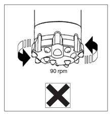
Rotating the bit faster than necessary will not generally increase penetration speed but it will increase the wear rate, particularly in abrasive rock.
