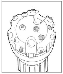
A DTH button bit can continue to drill with one or more broken buttons, but at a reduced penetration rate. Broken buttons should be ground off to prevent additional button particles breaking off and damaging other buttons.
