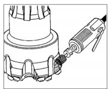
Ensure that the flushing holes are not deformed and grind them if necessary.
