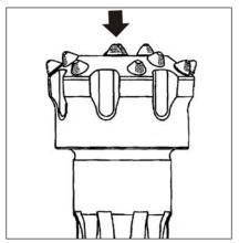
Broken inserts are generally caused by overdrilling the drill bit before reconditioning, reaming the hole, using excessive feed force or where there are existing tungsten carbide or other metal particles in the hole.
