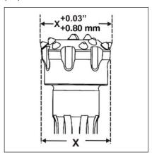
In highly abrasive conditions, the metal may wear more quickly than the carbide inserts. This is known as 'body wash' and in order to minimise carbide breakages, the carbide should be ground so that it does not protrude more than 9 mm (0.35") above the metal surface.
