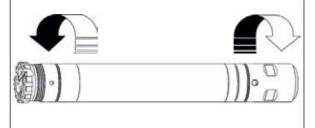
**C.** Unscrew and remove Drill Bit, Chuck (19), Chuck Spacer (16) and Bit Retaining Rings (15) from bottom of Cylinder (12).
