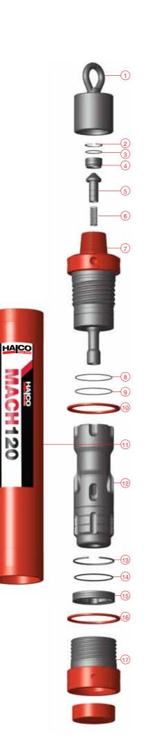
D. Remove Chuck Spacer (16) from Chuck (17). Remove Bit Retaining Rings (15) from Drill Bit and remove Containment Band (14) from Bit Retaining Rings (15).
