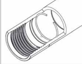
**D.** Fit 'O' Ring (14) to Bit Guide Bush (15) ensure it seats in the 'O' ring groove. Insert Bit Guide Bush (15) into bottom of Cylinder (12) ensure it seats up against Snap Ring (13).
