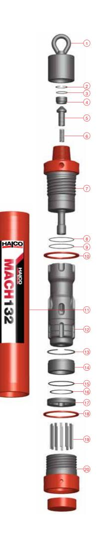
D. Remove Chuck Spacer (18) from Chuck (20). Remove Bit Retaining Rings (17) from Drill Bit and remove Containment Band (16) from Bit Retaining Rings (17). E1. MACH 132 VERSIONS Remove Chuck (20) and Drive Pins (19) from Drill Bit. CIE: **E2. MACH 142 VERSIONS** Remove Chuck (20) and Drive Pins (19) from Drill Bit. F. Remove 'O' Ring (15) from bottom of Cylinder (11). G. Remove Bearing Bush (14) from bottom of Cylinder (11).
