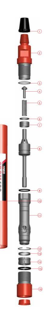
F. If required fit Containment Band (13) onto Bit Retaining Rings (14). Fit Bit Retaining Rings (14) onto Drill Bit.
