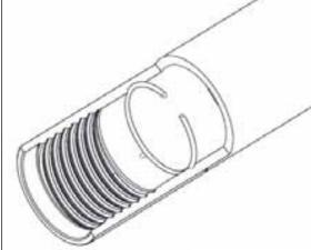
**D.** Grease splines and fit Chuck (15) onto Drill Bit.
