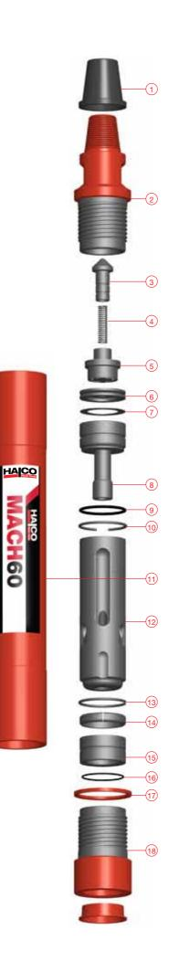
D. Remove Chuck Spacer (17) from Chuck (18). Remove Bit Retaining Rings (15) from Drill Bit and remove 'O' Ring (16) from Bit Retaining Rings (15). E. Remove Chuck (18) from Drill Bit. F. Remove Bottom Spacer (14) from Cylinder (11). G. Remove Snap Ring (13) from the bottom of Cylinder (11) using the tools illustrated below. Snap Ring Removal Tool Lever type part No. 601642 Snap Ring Removal Tool Hook type part No. 601574
