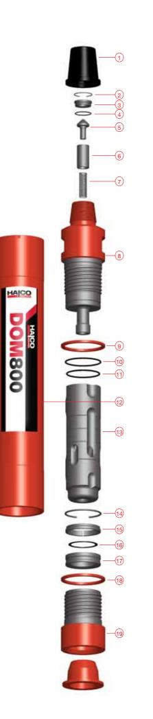
D. Remove Chuck Spacer (18) from Chuck (19). Remove Bit Retaining Rings (17) from Drill Bit and remove Containment Band (16) from Bit Retaining Rings (17). E. Remove Chuck (19) from Drill Bit. F. INGERSOLL RAND VERSIONS ONLY Remove Spacer (15) from Cylinder (12). G. Remove Snap Ring (14) from Cylinder (12) using the tools illustrated below. Snap Ring Removal Tool Lever type part No. 601642 Snap Ring Removal Tool Hook type part No. 601574 H. Remove Piston (13) from bottom of Cylinder (12).
