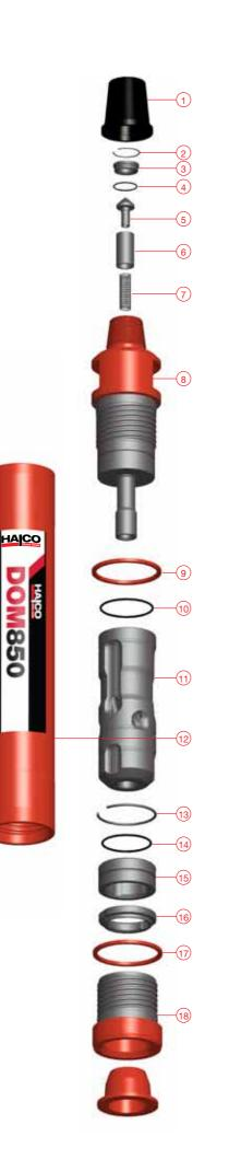
**E.** Grease splines and fit Chuck (18) onto Drill Bit. F. Fit Chuck Spacer (17) onto Chuck (18), Fit Bit Retaining Rings (16) over Drill Bit and insert into Chuck (18). **G.** Grease threads and screw Drill Bit, Chuck (18), Chuck Spacer (17) and Bit Retaining Rings (16) into bottom of Cylinder (12). H. Coat Piston (11) liberally with rock oil, minimum 200 centistroke and insert into top of Cylinder (12) ensure it is facing the right way as illustrated.
