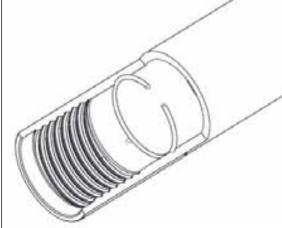
**D.** Fit Chuck Lock Ring (15) onto Chuck (17). Grease splines and fit Chuck (17) onto Drill Bit.
