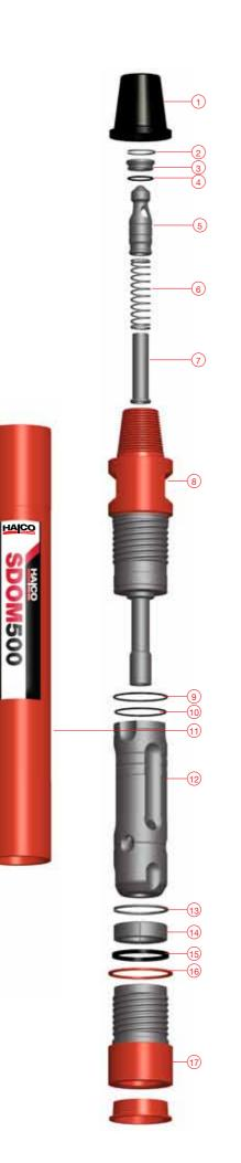
U ğ **D.** Remove Chuck Spacer (16) from Chuck (17) and remove Bit Retaining Rings (14) from Drill Bit. E. Remove Chuck (17) from Drill Bit and remove Chuck Lock Ring (15) from Chuck (17) if fitted. F. Remove Snap Ring (13) from Cylinder (11) using the tool illustrated below. Snap Ring Removal Tool Lever type part No. 601642 Snap Ring Removal Tool Hook type part No. 601574 (8). G. Remove Piston (12) from Cylinder (11).
