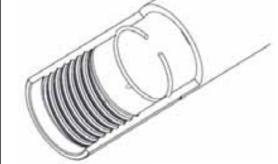
**D.** Insert Spacer (15) into the bottom of Cylinder (13) ensure it seats fully up against Snap Ring (14).
